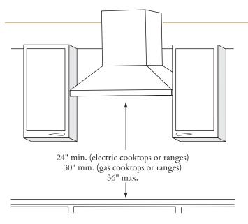
For the installation at left, conceal the ductwork running from the top of the hood. Use of the duct cover requires special consideration to the installation height above the countertop.
