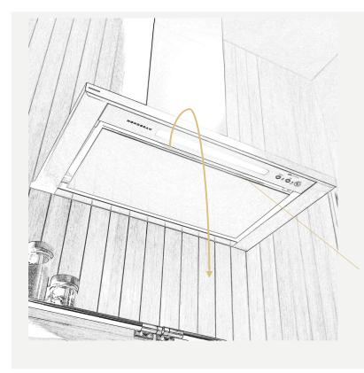
1. Swing open perimeter panel, which is the large rectangular door on the bottom of the hood
