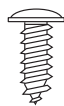
6 Phillips head screws to secure hood to the wood support: (2 secured to wood support)
