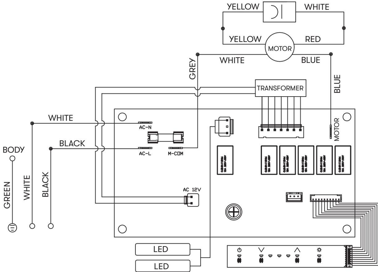
REMARKS: CONDENSER 3uF 250V AC FIT AC120V 60Hz
