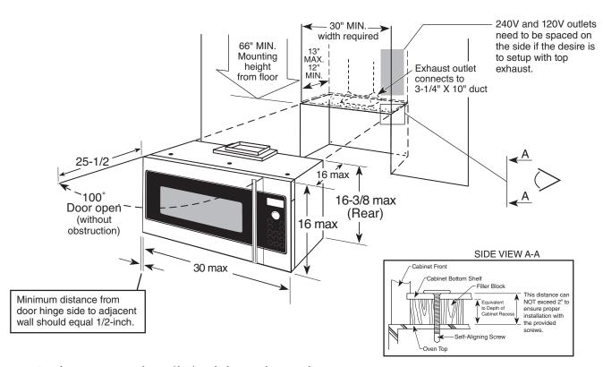
Note: Outside venting is optional. Vent (duct) can be horizontal or vertical.
