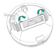
4 Reinstall the multi-surface brush and brush cover in the robot.
