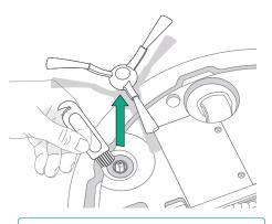
IMPORTANT: It is recommended to replace the edge sweeping brush every 3-6 months for an optimal cleaning effect.
