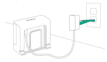
Plug the power cord into the wall. Wrap the cord back so it won't get in the way of the robot as it comes and goes.
