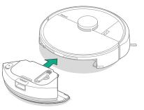
7 Place robot back on dock and use app or robot buttons to start cleaning.
