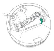
**3** Remove any hair and debris from the multisurface brush using the cleaning brush.
