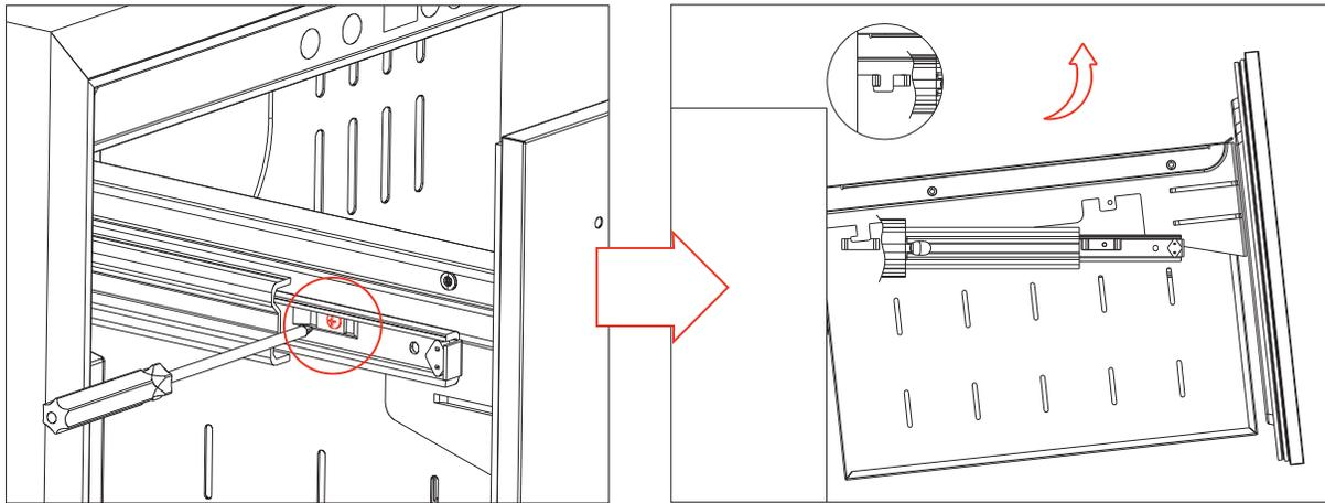
1. Remove the screw holding each slide rail and drawer bracket with a screwdriver
