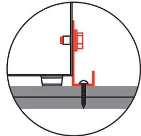
**CONCRETE FLOORING:** (Expansion Bolt) A 3/8" hole is bored into the flooring 1 3/4" to 2" deep. The expansion sleeve is set with a mallet into the hole and the bracket is bolted to the floor.
