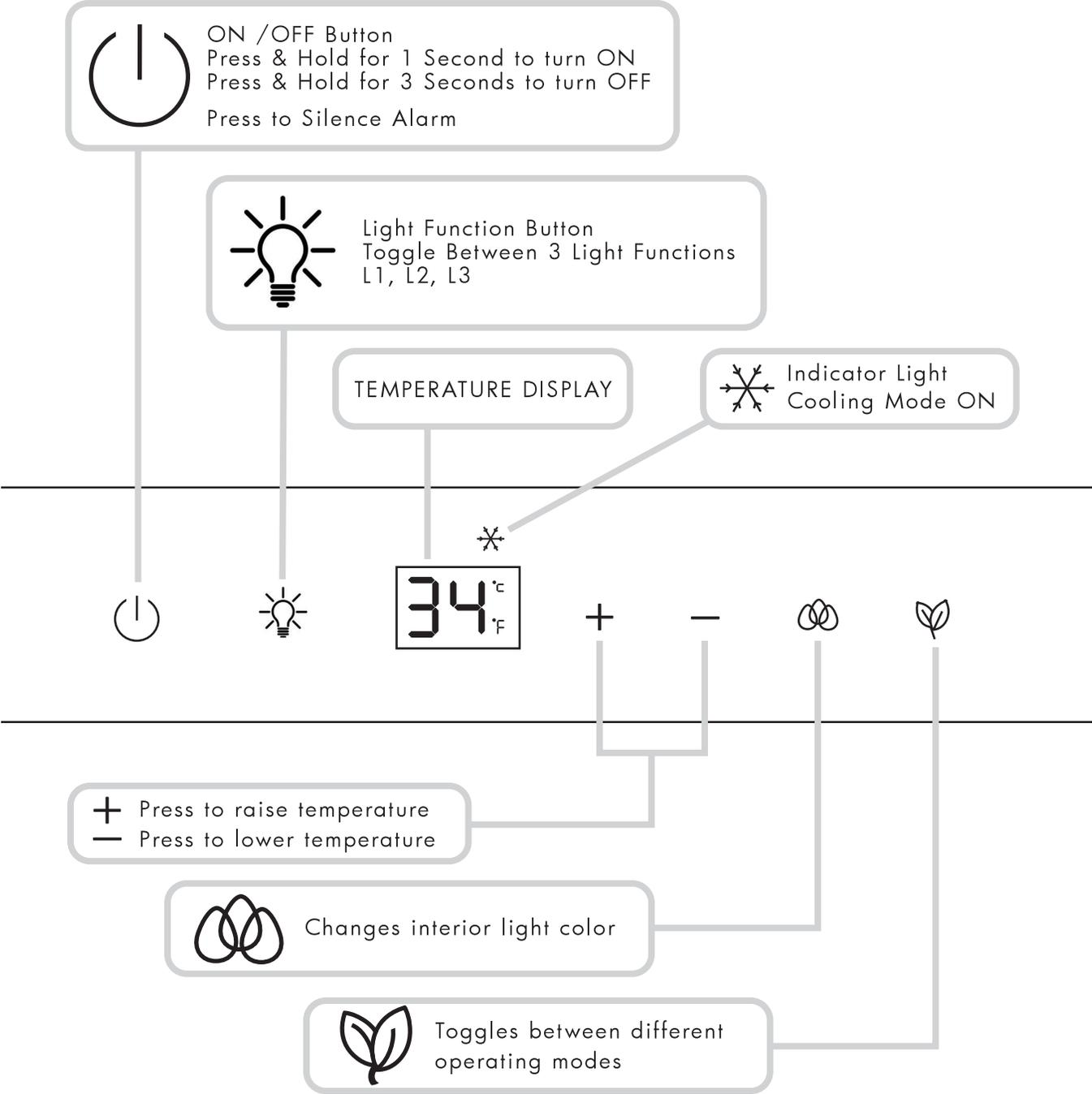
The temperature setting can be adjusted from 34-50°F.
