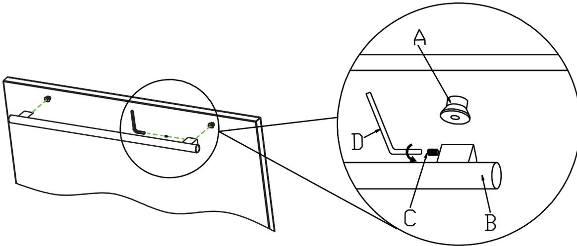
Push the handle tightly against the door and tighten both of the 2 set screws (C) with the hex key (D).
