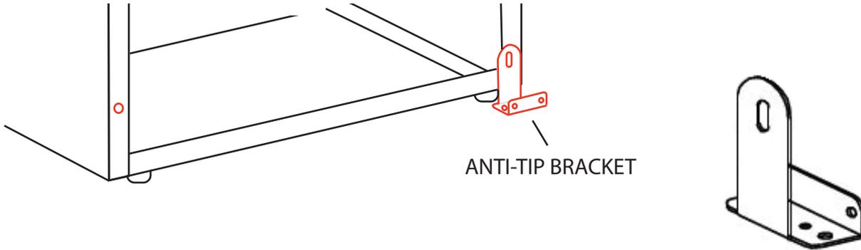
The Anti-Tip Bracket kit comes with a bolt and washers to mount to the rear of the refrigerator and three different sets of fasteners to mount it to any of the following: Dry Wall Construction, Wooden Flooring or Concrete Flooring.
