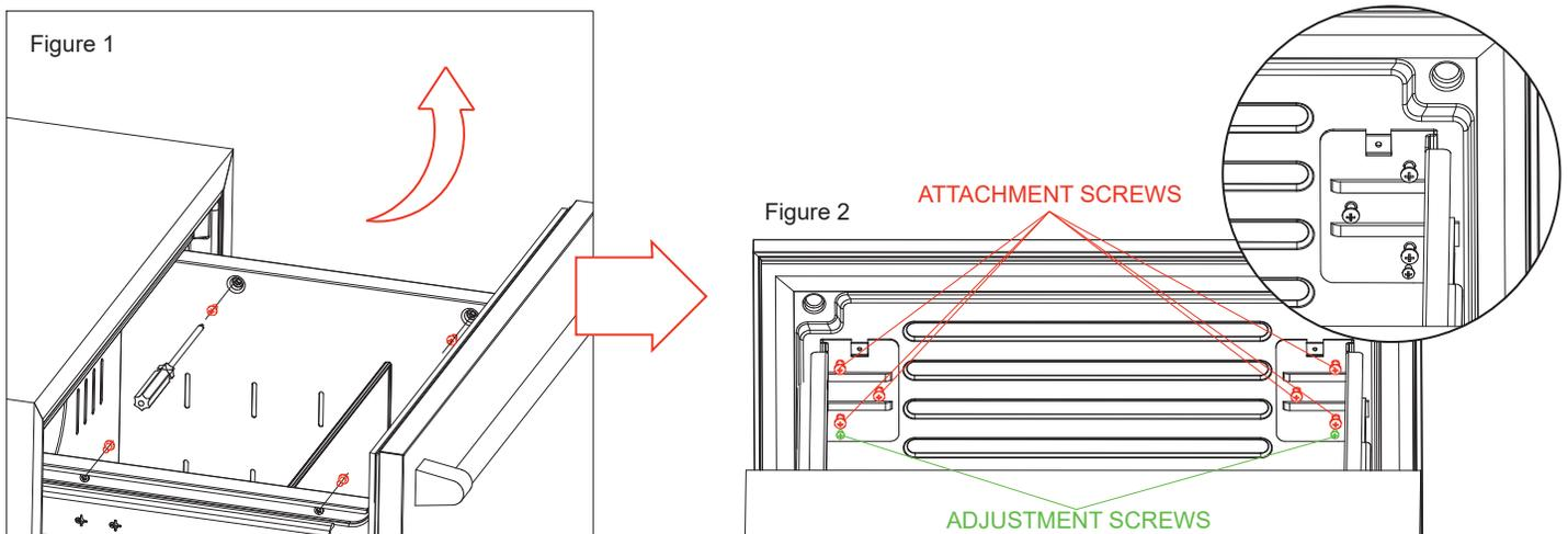
1. Remove the drawer from the side rails by removing the four screws shown in Fig 1
