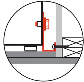
**WOODEN FLOORING:** (2 Screws) The bracket must be screwed down into the flooring.
