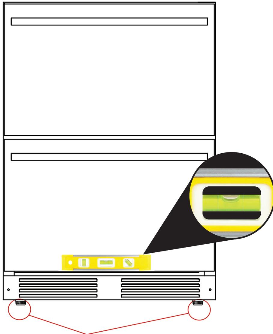
Rotate to raise or lower the **LEVELING LEGS** located at each of the four corners until all four legs are seated firmly on the floor and the interior floor of the unit is level **both front to back and side to side**.
