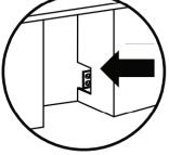
TIP: IN TIGHT INSTALLATIONS CUT THROUGH AN ADJACENT CABINET WALL TO REACH AN OUTLET INSTALLED THERE
