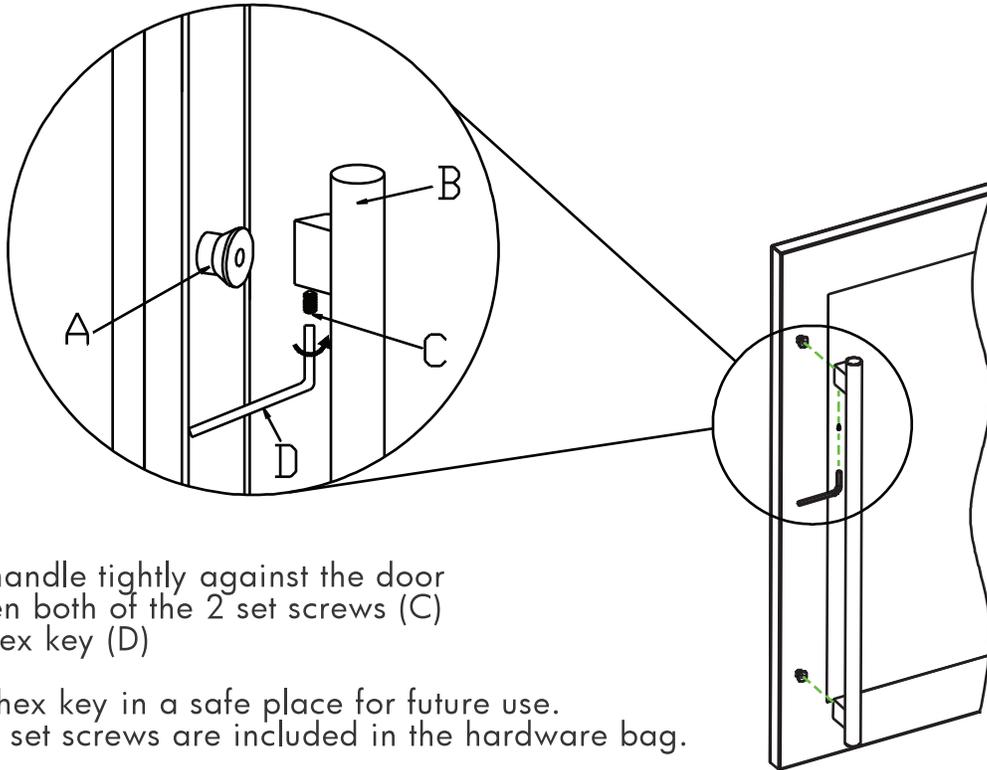
Push the handle tightly against the door and tighten both of the 2 set screws (C) with the hex key (D)
