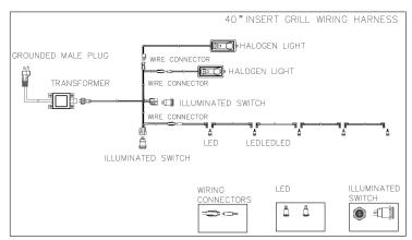
NOTE: To install the electrical transformer to the cart use the 4 Bolts provided in your hardware pack. The transformer has 4 holes that will match up to the holes on the back panel of the cart. face the transformer main electrical wire "facing down" and the wire from the gas grill will connect securely into the top of the transformer making a watertight fit.
