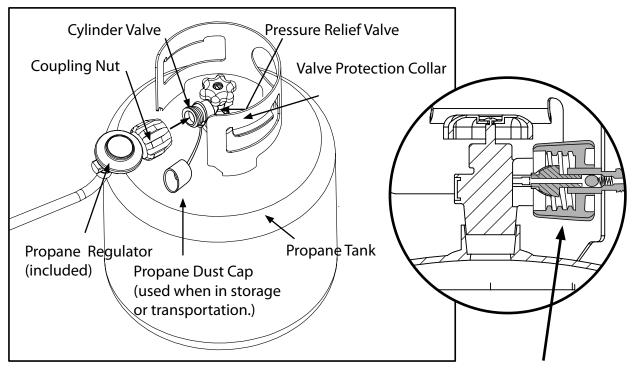
Hand tighten to ensure proper seal for correct gas flow.
