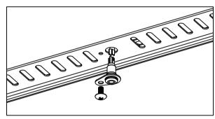
Remove the lock nut and light holder from the old bulb.
