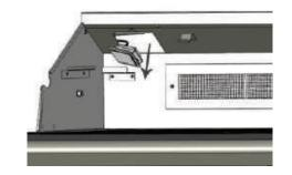
With the light cover removed pull the halogen bulb out sideways from light socket.
