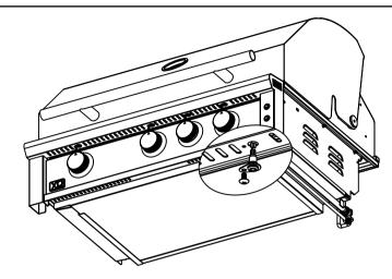
Remove the LED light assembly and disconnect it from the power connector.
