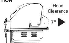
No materials shall be used within 12" of the unit that will burn or be affected by the high heat the unit can produce.
