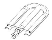
The performance series stainless U-Style XLT burner is used in this XO gas grill. This new burner has even heat distribution that enables rapid heating throughout the cooking area.
