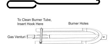
For safe operation ensure the Gas Valve Assembly Orifice is inside the Burner Tube before using your grill. (See figure above). If the Orifice is not inside the Burner Tube, lighting the Burner may cause explosion and/or fire resulting in serious bodily injury and/or property damage.
