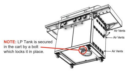
The grill cart has air vents on three sides to allow for the release of excess vapor.
