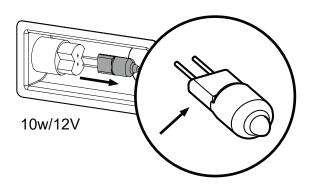
Replace bulb by pushing it straight into light socket. Re-attach light cover, and reinstall housing repeating steps 2. and 3. in reverse order.
