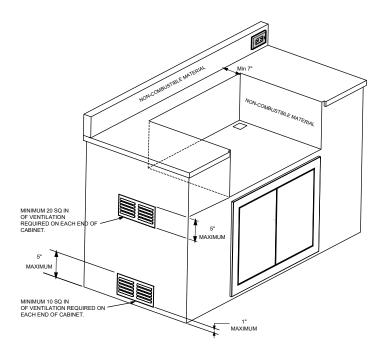
A minimum of three 10 in<sup>2</sup> (65 cm<sup>2</sup>) of ventilation openings must be provided at the bottom of the back, left and right sides of your enclosure (island).
