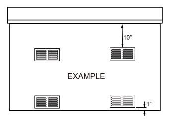
Natural Gas is lighter than air. Vents should be placed 10" below the countertop.
