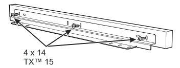
Mount the panel onto the angle bracket using three 4 x 14 screws.
