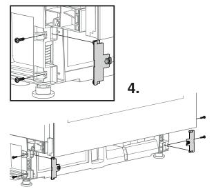
5. Fit the adjustable feet **7.** support. 4 x 29 TX™ 15 7. • Screw the appliance to the body of the cabinet at the top left-hand side. • Click cover (1) into place 5. again. Screw the appliance to 6. the body of the cabinet at Slide in the appliance the bottom on the left and until the front surface right. of the appliance door is flush with the cabinet fronts. 8. **⚠** WARNING! I 4 x 29 TX™ 15 4 x 29 TX™ 15 When sliding in the appliance, make sure
