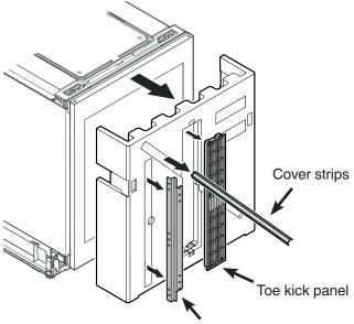
Angle bracket (for mounting a cover panel on the top or bottom of the appliance)
