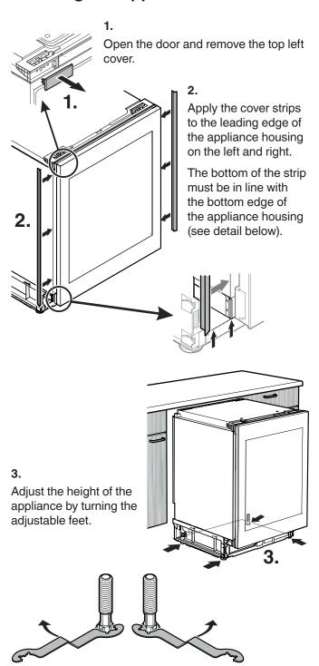
Turn the wrench counterclockwise to raise the appliance and clockwise to lower it. Position the wrench accordingly.
