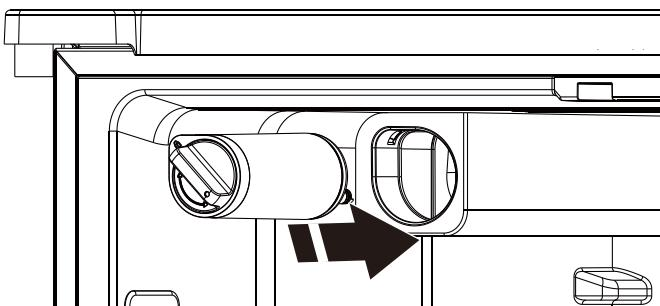
5. Turn the locking knob clockwise 180° to keep the filter locked.
