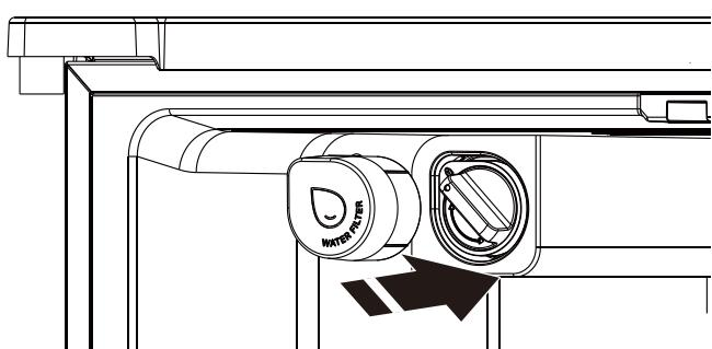
4. Pick up the new filter and remove the shield from the filter.
