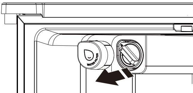
2. Turn the locking knob 180° counterclockwise so that the filter is in the non-locking state.
