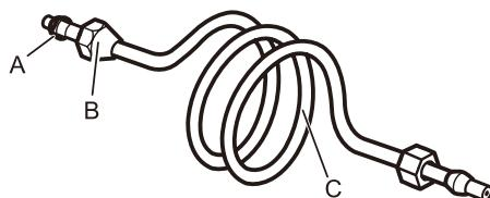
A. Compression sleeve      C. Copper tubing
