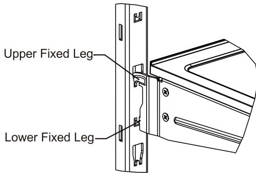
**NOTE:** Hole 1 can only be used for left half shelf support, and Hole 2 can only be used for right half shelf support, if placed incorrectly, the shelf will be unstable and can not be used.
