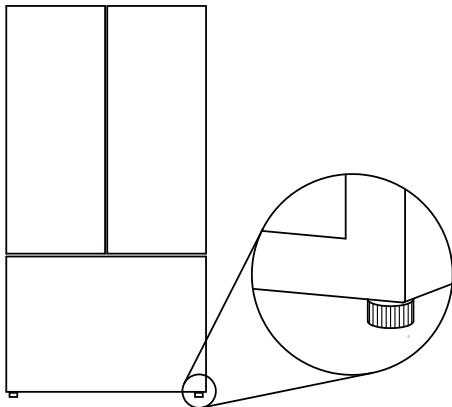
4. Use a household tool to lift the refrigerator up as required. This will make adjusting leveling legs easier.
