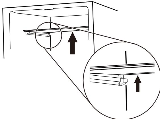
2. Move the glass shelf forward and lower the front shelf down until the rear trim is out of supports.
