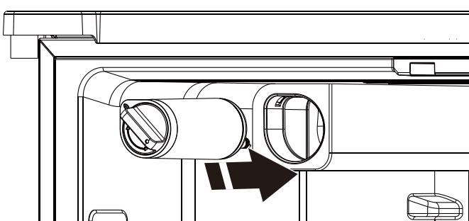
7. Turn the locking knob clockwise 180° to keep the filter locked.
