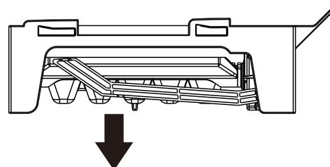
**NOTE:** Turn off the ice maker before removing the ice storage bin to serve ice or to clean the bin. This will keep the ice cubes from dropping out of the ice maker and into the freezer compartment. After replacing the ice storage bin, turn on the ice maker.
