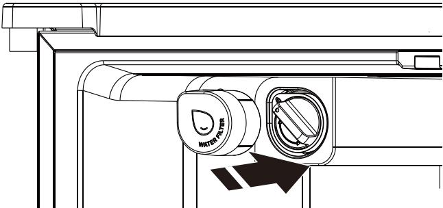
**NOTE:** If the filter is not installed correctly, water may dispense at a lower flow rate and there will be slower ice production. Improper filter installation may also cause the water filter housing to leak.
