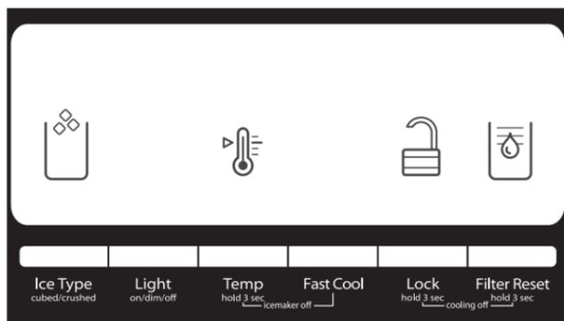
For your convenience, your refrigerator and freezer controls are preset at the factory. When you first install your refrigerator, make sure that the controls are still set to the "mid-settings." The factory recommended set points are 38°F (3°C) for the refrigerator and 0°F (-18°C) for the freezer.
