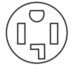
4-wire receptacle (14-30R)
