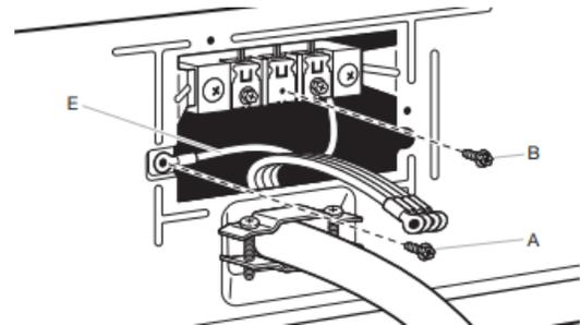
Remove center terminal block screw (B). Remove neutral bond wire (E) from green external ground conductor screw (A).
