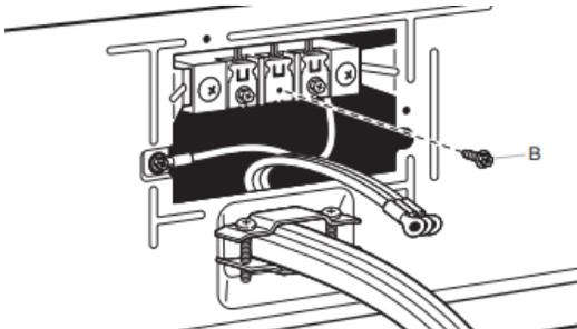
Remove center terminal block screw (B).
