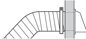
Vent must fit over the exhaust hood. Secure vent to exhaust hood with 4" (102 mm) clamp. Run vent to dryer location using straightest path possible. Avoid 90° turns. Use clamps to seal all joints. Do not use duct tape, screws, or other fastening devices that extend into interior of vent to secure vent, because they can catch lint.
