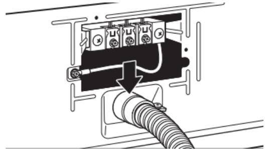
Put direct wire cable through the strain relief. The strain relief should have a tight fit with the dryer cabinet and be in a horizontal position. Tighten strain relief screw against the direct wire cable.
