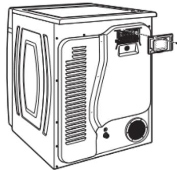
Remove hold-down screw and terminal block cover.
