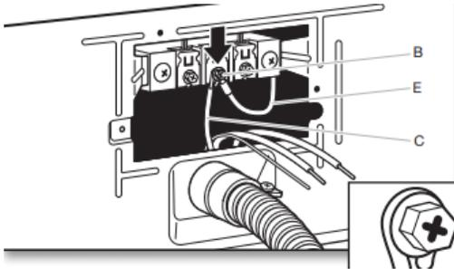
Connect neutral bond wire (E) and place hooked end (hook facing right) of neutral wire (white or center wire) (C) of direct wire cable under center screw of terminal block (B). Squeeze hooked ends together and tighten screw.
