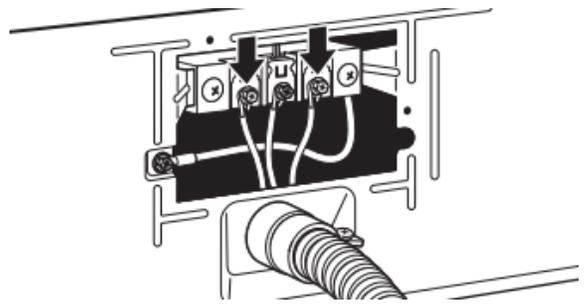
Place hooked ends of remaining direct wire cable wires under outer terminal block screws (hooks facing right). Squeeze hooked ends together and tighten screws. Insert tab of terminal block cover into slot of dryer rear panel. Secure cover with hold-down screw. Now, go to "Venting Requirements."
