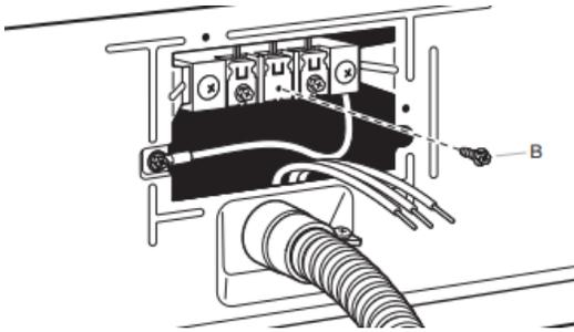
Remove center terminal block screw (B).
