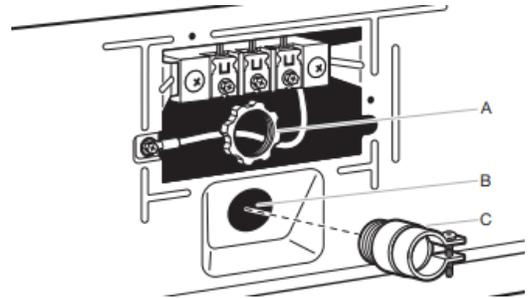
Unscrew the removable conduit connector (A) and any screws from a 3/4" (19 mm) UL-listed strain relief (UL marking on strain relief). Put the threaded section of the strain relief through the hole below the terminal block opening (B). Reaching inside the terminal block opening, screw the removable conduit connector (A) onto the strain relief threads (C) and tighten securely.
