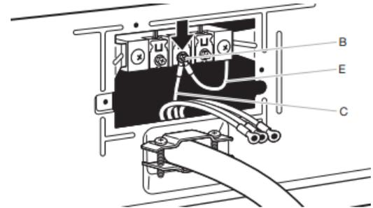
Connect neutral bond wire (E) and neutral wire (white or center) (C) of power supply cord under center terminal block screw (B). Tighten screw.
