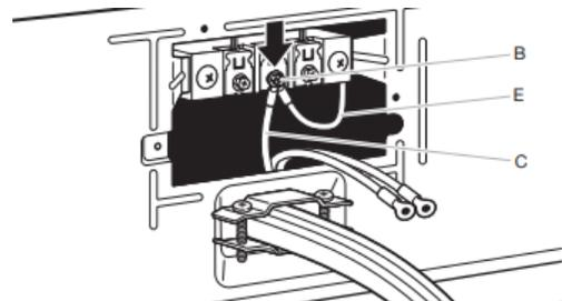
Connect neutral bond wire (E) and neutral wire (white or center) (C) of power supply cord or cable under center terminal block screw (B). Tighten screw.
