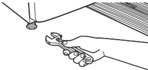
If dryer is not level, prop up using a wood block. Use wrench to adjust legs up or down, and check again for levelness.
