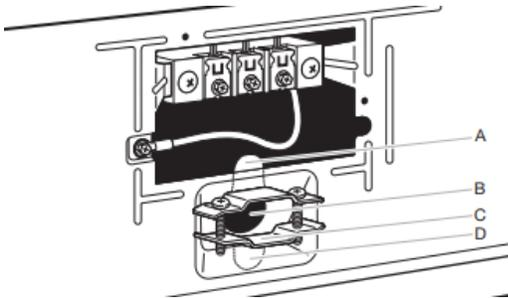
Remove the screws from a 3/4" (19 mm) UL-listed strain relief (UL marking on strain relief). Put the tabs of the two clamp sections (C) into the hole below the terminal block opening (B) so that one tab is pointing up (A) and the other is pointing down (D), and hold in place. Tighten strain relief screws just enough to hold the two clamp sections (C) together.
