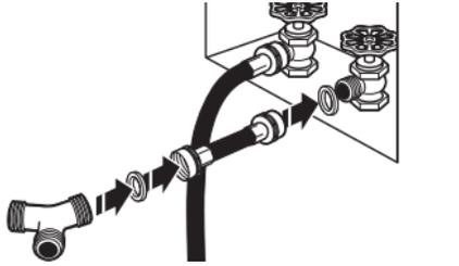
Attach 2 ft (0.6 m) inlet hose to cold water faucet. Screw on coupling by hand until it is seated on faucet. Then attach “Y” connector to male end of the 2 ft (0.6 m) inlet hose. Screw on coupling by hand until it is seated on connector.
