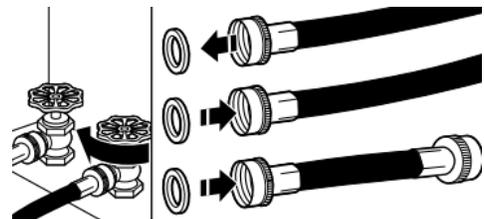
Turn cold water faucet off and remove washer inlet hose. Remove old rubber washer from inlet hose and replace with new rubber washer.
