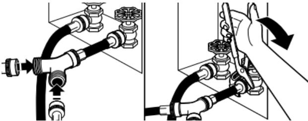
Attach one of the 5 ft (1.5 m) inlet hose ends to the “Y” connector. Attach washer cold inlet hose to other side of “Y” connector. Screw on coupling by hand until it is seated on connector. Using pliers, tighten the couplings an additional two-thirds turn.
