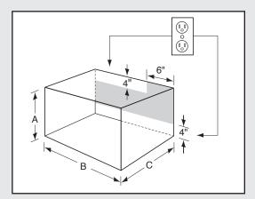
The built-in trim kit includes all the necessary parts and easy-to-follow instructions for installation as well as location of the power supply.
