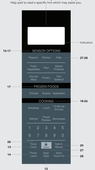
The two-line, Interactive Display spells out operating steps and shows cooking hints. When HELP is lighted in the display, touch the Help pad to read a specific hint which may assist you.
