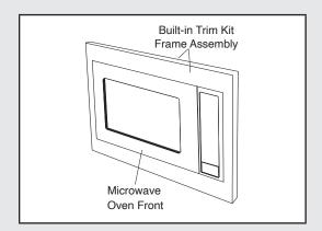
See built-in trim kit installation instructions for proper location when building in above the specified ovens. Carefully follow both the oven installation instructions and built-in trim kit instructions.
