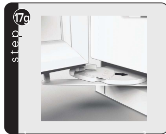
Remove spacer adjustment tool by sliding it back from bushing
