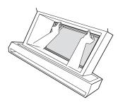
Hold the top of the auto-lift device with both hands and remove it from the bottom drawer.
