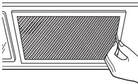
**7** Install grease filters. See the Use and Care packed with the microwave.
