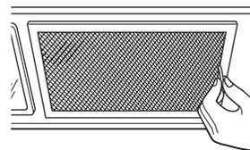
**8** Install grease filters. See the Use and Care packed with the microwave.
