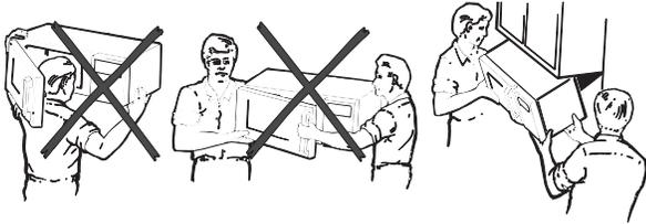
POUR VOTRE SÉCURITÉ ET POUR FACILITER L'INSTALLATION, L'INSTALLATION DE CE FOUR DOIT ÊTRE EFFECTUÉE PAR DEUX PERSONNES.
