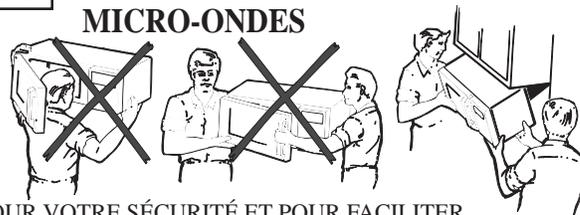
POUR VOTRE SÉCURITÉ ET POUR FACILITER L'INSTALLATION, L'INSTALLATION DE CE FOUR DOIT ÊTRE EFFECTUÉE PAR DEUX PERSONNES.
