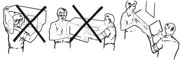
POUR VOTRE SÉCURITÉ ET POUR FACILITER L'INSTALLATION, L'INSTALLATION DE CE FOUR DOIT ÊTRE EFFECTUÉE PAR DEUX PERSONNES
