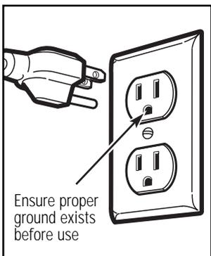
The power cord of this appliance is equipped with a three-prong (grounding) plug which mates with a standard three-prong (grounding) wall receptacle to minimize the possibility of electric shock hazard from this appliance.
