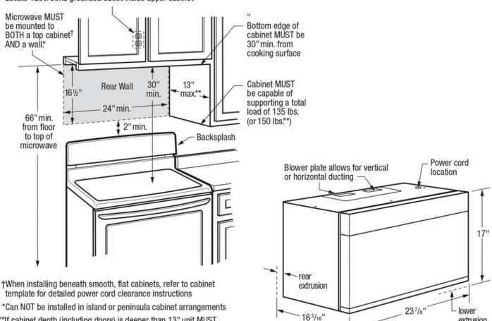
Locate 120V/60Hz grounded outlet inside upper cabinet
