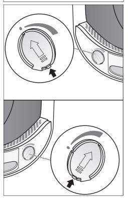
To open the cover, push the tab all the way up to the top.
