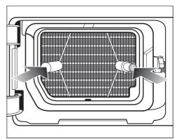
Push the plinth filter in completely.
