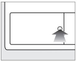
Press the round, indented area on the heat exchanger access panel to open it.
