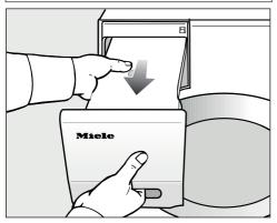
Remove the condensed water container.
