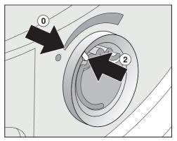
Turn the outer ring counterclockwise until marker (2) is in position (0).
