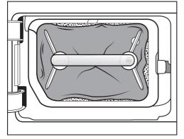
The edges of the plinth filter do not sit properly and the plinth filter is deformed. Lint will blow into the heat exchanger unfiltered through edges that do not sit properly. This will cause a permanent obstruction in the heat exchanger.
