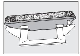
Residues arise from laundry fibers and traces of detergent components. They can be found on the front and side edges of the plinth filter. In extreme cases, they can form stubborn crust. Residues are a sign that the plinth filter no is longer a snug fit at the sides, even if it appears to be perfect:
