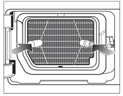
■ Push the plinth filter in completely.
