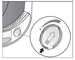
■ To open the cover, push the tab all the way up to the top.
