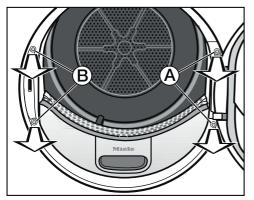
Use a T30 Torx screwdriver to unscrew the two screws on the base plate of the door hinge (A).
