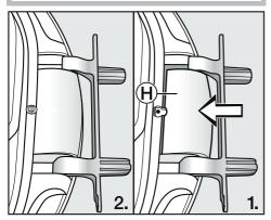
■ Fit new door hinge cover (H) and clip it into position.
