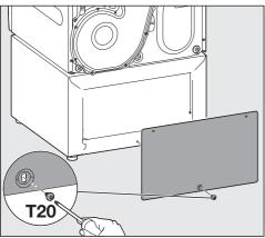
Screw the rear panel onto the base at the bottom using one of the raised head screws provided so it is handtight.
