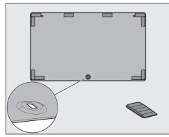
Stick the sealing strips from the accessory pack to the inside of the rear panel as shown in the image.
