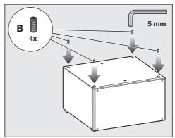
Screw the shorter set screws B all the way into the base.
