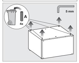
■ Unscrew set screws **A** using an Allen wrench.
