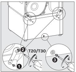
Use the raised head screws to screw the connecting pieces and the rear panel to the base.
