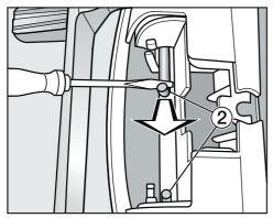
Use the screwdriver or pointed pliers to guide first one then the other rod
