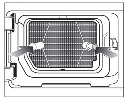
■ Push the plinth filter in completely.
