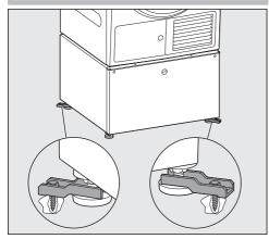
Anchor the base feet diagonally with the tensioning strips provided, e.g., the front right foot and the rear left foot.
