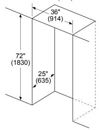
Leave  $\frac{1}{2}$ " (12.7) gap at the top and 1" (25.4) behind the refrigerator for proper ventilation.
