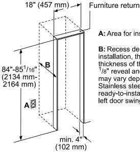
**A:** Area for installation of power connection.
