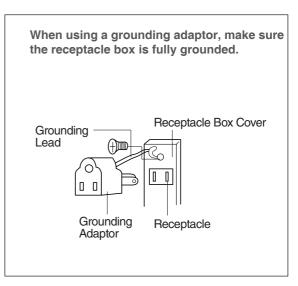
"THE CANADIAN ELECTRICAL CODE DOES NOT ALLOW THE USE OF THE GROUNDING ADAPTOR"
