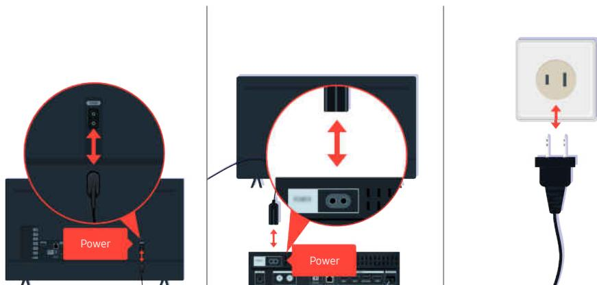
First disconnect and reconnect the power cables and HDMI cables on the back of your TV or the One Connect Box, then unplug the power cord and plug it back into the wall outlet.
