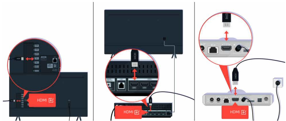
Check the antenna and HDMI cable connections.
