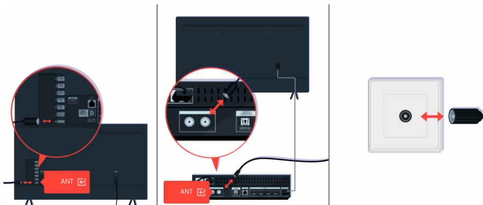
Check the antenna and input cable connections.
