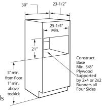
• Oven overlaps will conceal cut edges on all sides of the opening. **Note:** PSB9120 series Advantium can be installed below GE/GE Profile non-downdraft gas and electric cooktops. It CANNOT be installed below induction or Monogram (2GU3841385) gas cooktops.
