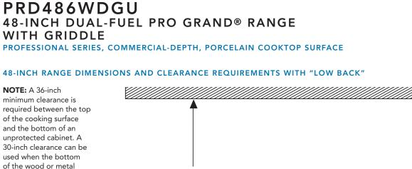
unprotected cabinet. A 30-inch clearance can be used when the bottom of the wood or metal cabinet is protected by not less than 1/4 inch of a flame retardant material covered with not less than No. 28 MSG sheet steel, 0.015 inch (0.4 mm) thick stainless steel, 0.024 inch (0.6 mm) aluminum, or 0.020 inch (0.5 mm) thick copper.
