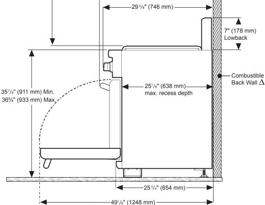
$\Delta$  As defined in the "National Fuel Gas Code" (ANSI Z223.1, Current Edition). Clearances from non-combustible materials are not part of the ANSI Z21.1 scope and are not certified by CSA. Clearances of less than 6" (152 mm) must be approved by the local codes and/or by the local authority having jurisdiction.
