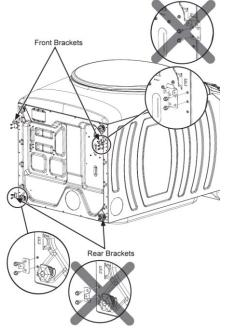
• Install the rear brackets on the bottom of the Combo. Use the top 2 holes on the bottom of the Combo with the tab on the bracket facing the outside.
