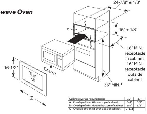
\*For ADA compliance, the microwave must be installed no higher than 37-7/8".
