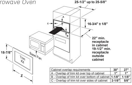
NOTE: Allow an additional inch of clearance beyond trim kit frame on all sides to prevent the trim kit from blocking any outside adjoining cabinets/obstructions. Reference below drawing.
