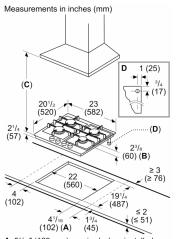
A: 5¹/₁₅" (129 mm) required when installed with a built-in oven
