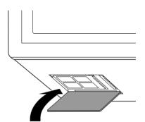
4 To reinstall the grease filter, insert the back of the filter, push the filter toward the back, and lift the filter up into place.
