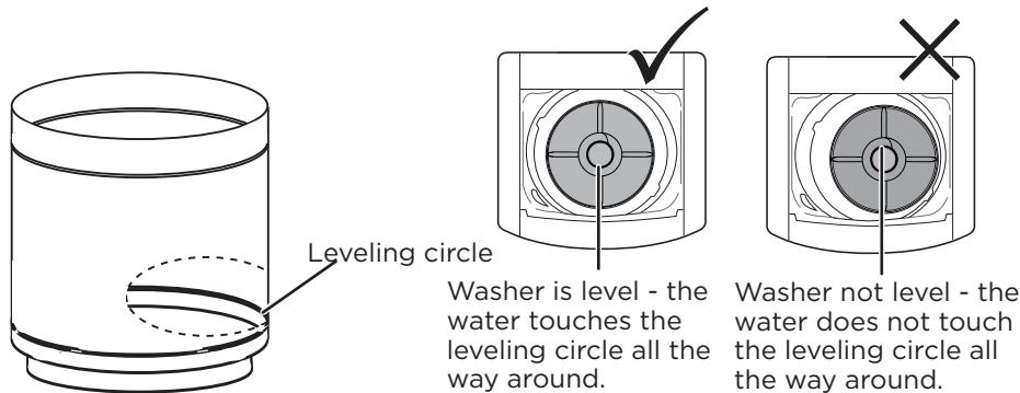
3. If your washer is not level, carefully tilt your washer just enough to adjust the leveling feet on the bottom front of your washer. Extend the feet only as much as is necessary. If the feet are extended too much, your washer may vibrate
