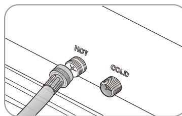
**NOTE:** If you do not want to use the hot water supply hose, insert a water intake cap into the hot water supply intake hole. In this case you must select the Tap Cold option for the water temperature.
