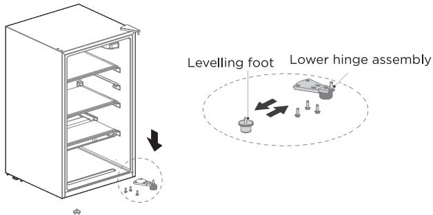
4. Install the door on the lower hinge assembly, and then install the upper hinge, hinge cover, shaft sleeve, pins and hole cap in sequence.
