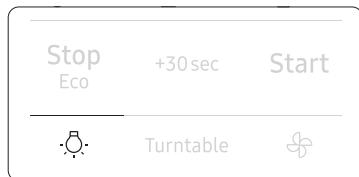
Touch the button to turn the cooktop lamp on or off. Touch the button once for high, twice for low, and three times to turn the cooktop lamp off.
