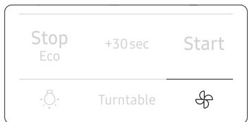
Touch the button once for high fan speed, twice for medium fan speed, and three times for low fan speed. Touch the button four times to turn the fan off.
