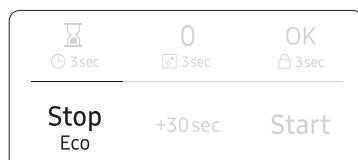
Eco Mode reduces standby power usage. When you touch the **Stop/Eco** button once, the display will go out and the microwave shifts to a mode which minimizes power usage. To cancel the Eco Mode, touch any other button.
