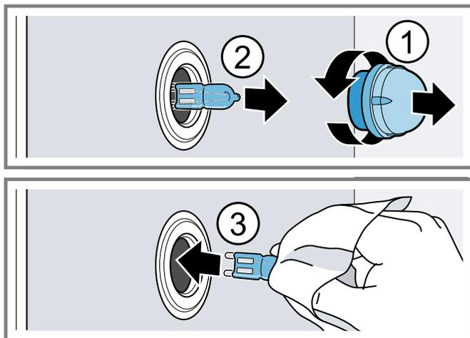
4. Remove the old bulb by grasping and sliding the bulb straight back until the two prongs have cleared the ceramic holder ②.
