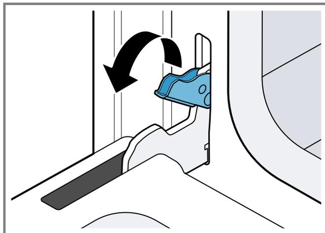
If necessary, use a tool, such as a screwdriver, to gently pry the upper part of the lever away from the housing. Take care to avoid scratching the housing.
