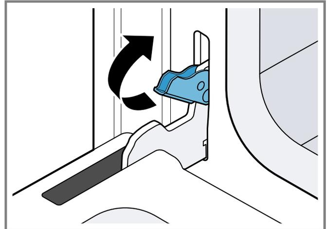
6. Close and open the door slowly to be sure it is correctly and securely in place.
