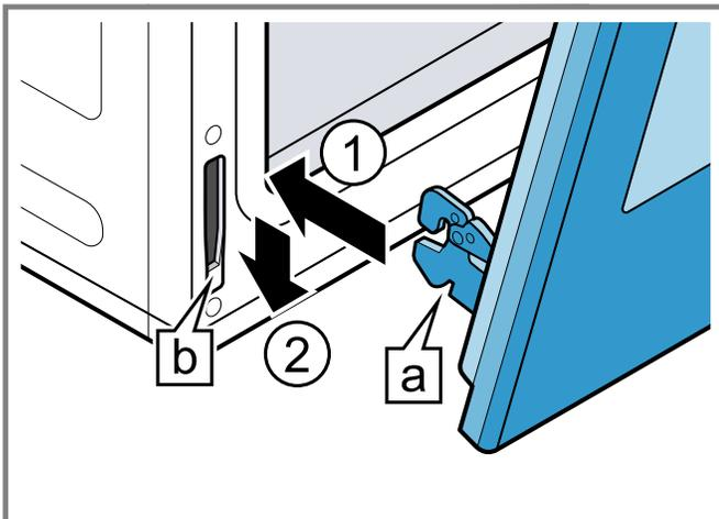
The angle of the door may need to be adjusted slightly to allow the hinges to engage properly and the door to lower into place. The door should lower about 3/4" (2 cm) and stop. If it does not, the hinges have not engaged properly and the door could fall if it is released.
