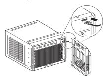
Attach the front grille to the cabinet by inserting the tabs on the grille into the slots on the front top of the cabinet.
