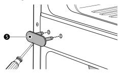
Remove the decorative screw 6 located on the housing between the freezer and refrigerator doors. (You will need this hole for the middle hinge bracket.)
