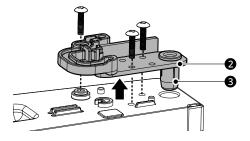
6 Move the bracket to the opposite side of the door and insert the hinge pin sleeve. Reverse the hinge lever ② by flipping it over. Place it on top of the bracket, and tighten both down with the screw. Then insert the remaining 2 screws to tighten the bracket to the refrigerator door.
