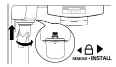
**5** After the water filter is replaced, dispense 2.5 gallons of water (flush for approximately 5 minutes) to remove trapped air and contaminants from the system.
