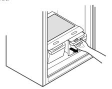
To reassemble, slightly tilt up the front of the crisper, insert it into the frame, and push it back into place.
