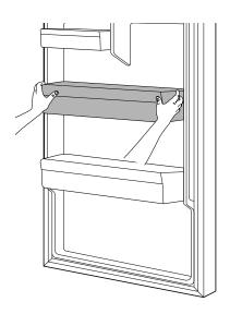
To assemble the bin, slide it in above the desired support and push down until it snaps into place.
