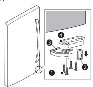
5 Turn the hinge lever 1 over and install it, the hinge bracket 2, screws 3, and hinge pin sleeve 4 on the bottom left side of the door.
