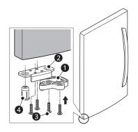
6 Use a 1/4 in. (6.35 mm) hex socket wrench to loosen the hinge pin 1 and remove it. Use a 3/16 in. (5 mm) Allen wrench and a Phillips screwdriver to remove the two Allen-head 2 and one Phillips-head 3 screws. Remove the hinge 4.
