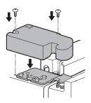
**15** Assemble the right hinge cap with the two screws.
