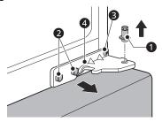
**7** With a flat-head screwdriver, carefully pry off and remove the cover over the bolt holes on the left side of the refrigerator.
