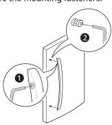
Carefully rotate the decorative screw covers 3 counterclockwise with your fingers until they loosen and fall out. Once they're removed, install the covers in the screw holes **4** on the opposite side.
