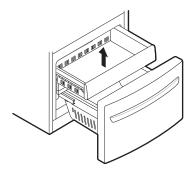
Remove the **Durabase** basket from the rails. Remove the screws from the rails at both ends.
