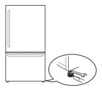
Open both doors, and check to make sure that they close easily. If the doors do not close easily, tilt the refrigerator slightly more to the rear by turning both leveling legs to the left. It may take several more turns, and be sure to turn both leveling legs the same amount.
