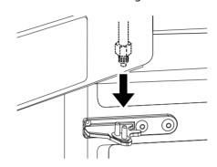
Fit the hinge **1** over the hinge lever latch **2** and slot it into place. Rotate the lever 3 clockwise and fasten the hinge.
