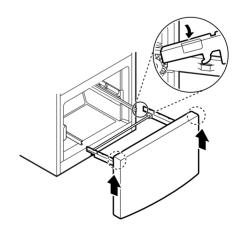
Lower the door into its final position and insert the screws in the rails on both sides.
