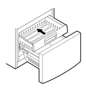
Replace the ice bin(s) in the drawer. Insert the Durabase basket in the rail assembly.
