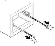
Grasp the drawer on each side and hook the drawer supports into the rail tabs located on both sides.
