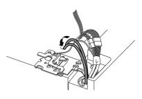
Hold the water supply connection and gently push in the collet **4** to connect the water supply lines as shown. Insert the tube at least 5/8 inch (15 mm) into the connector. Insert the clip on the joint to fasten the tubes in place.
