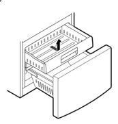
Remove the Durabase basket from the rails. Remove the screws from the rails at both ends.
