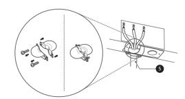
For conduit installations, insert the conduit strain relief in the 1 1/8 in. (2.8 cm) conduit hole. Then install the conduit through the body of the strain relief and fasten the strain relief with its ring.
