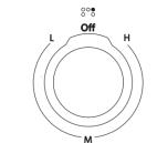
The control knobs can be set to anywhere between "H" and "L." Push in and turn to setting.
