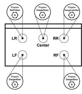
To prevent leakage, make sure the orifice spuds are securely screwed into the gas supply tubes.
