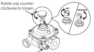
Lever shown open (Oven Shut Off only) PUSH LEVER DOWN TO CLOSE
