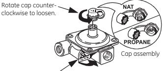
Lever shown closed (Öven Shut Off only) FLIP LEVER UP TO OPEN
