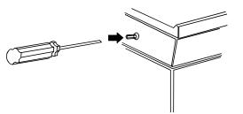
Center adjustment screw for all burners.
