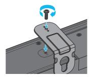
• When assembling, make sure the hanger part of the **Bracket-Wall Mounts** are located behind the rear of the Soundbar.
