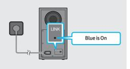
The LINK LED indicator stops blinking and glows a solid blue when a connection is established between the Soundbar and the Wireless Subwoofer.
