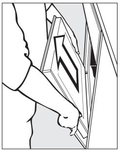
Hold the door on either side and pull it upwards off the hinge retainers. Make sure that the door is straight.
