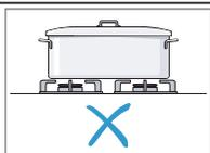
Never heat a cooking vessel (e.g. roasting tin, pan, cooking stone) with multiple burners, except for the griddle plate. The resulting accumulation of heat causes damage to the appliance.
