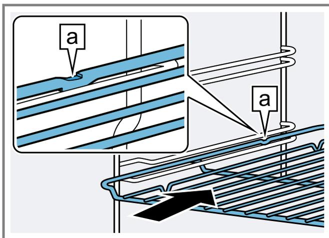
3. Tilt the rack up to allow the stop to slide onto the rack guide.
