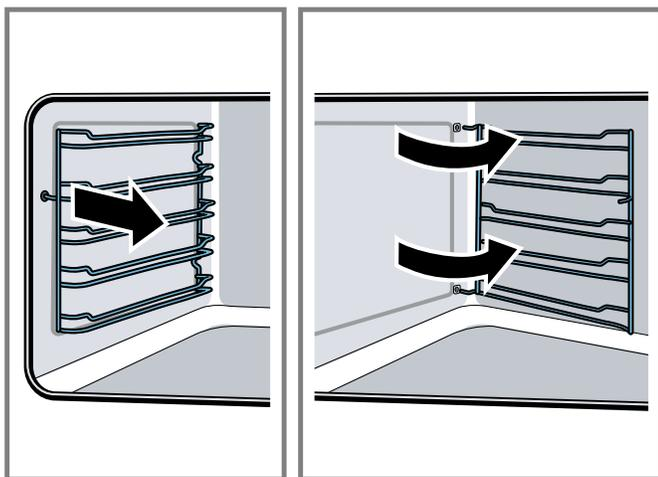
4. Replace the self-cleaning surfaces and rack guides in the reverse order in which they were removed.
