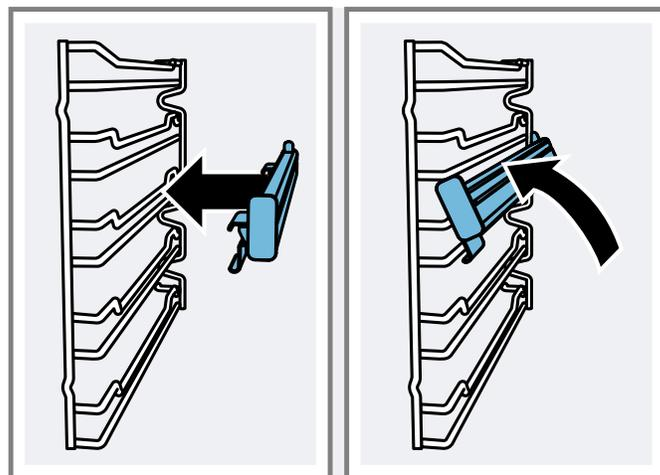
2. Clip the lower part of the rail onto the rack guide.
