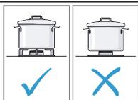
Place the pots on the pan supports, never directly onto the burners. Prior to use, ensure that the pan supports and lids of the gas burners are positioned correctly.
