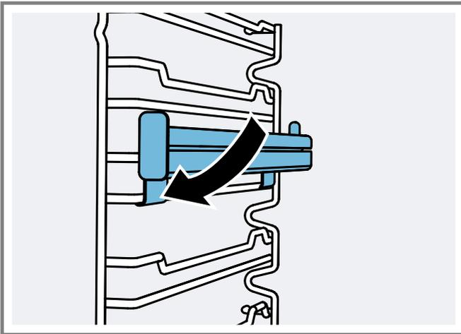
3. Slide the movable part of the telescopic rail in and out a few times to make sure it is able to move freely and that the stationary part of the telescopic rail is securely anchored.
