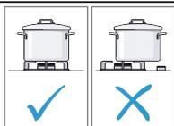
Place the cooking vessel in the center of the burner, otherwise it may tip over. Don't place large pots on the burners near the stove controls. They could overheat and become damaged.
