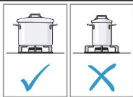
Use cooking vessels of appropriate size for the particular burner. Don't use small cooking vessels on large burners. The flame shouldn't come in contact with the sides of the cooking vessel.
