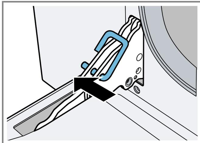
3. **⚠ CAUTION** Move the glass pane slowly to avoid damage to the glass and the oven cavity frame.
