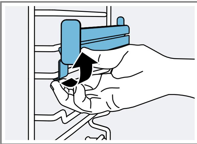
2. Lift the upper part of the rail off the rack guide.
