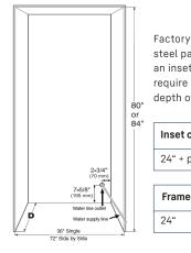
Factory available stainless steel panels are designed for an insetinstallation only and require a cabinet / gable depth of 24 - 3/4".
